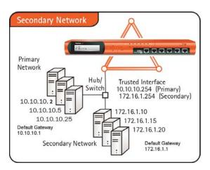
When you add a secondary network, you map an IP address from the secondary network to the IP address of the Firebox interface. Thus, you make (or add) an IP alias to the network interface. This IP alias is the default gateway for all the computers on the secondary network. The secondary network also tells the Firebox that there is one more network on the Firebox interface.
